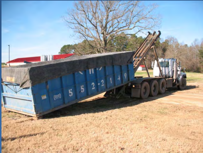
Roll-off of Dumpster
